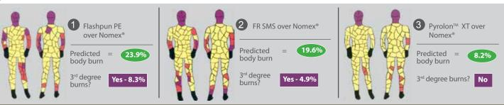
The testing shows that both standard disposables such as Flashpun and FR SMS garments result in higher predicted body burn with very little difference. Only Pyrolon™ garments result in a dramatic reduction in predicted body burn.
