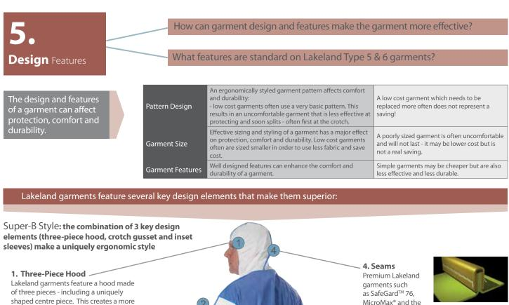
MicroMax® NS Cool Suit have stitched and bound seams featuring an additional strip of fabric wrapped around the seam, improving protection, strength and durability.
