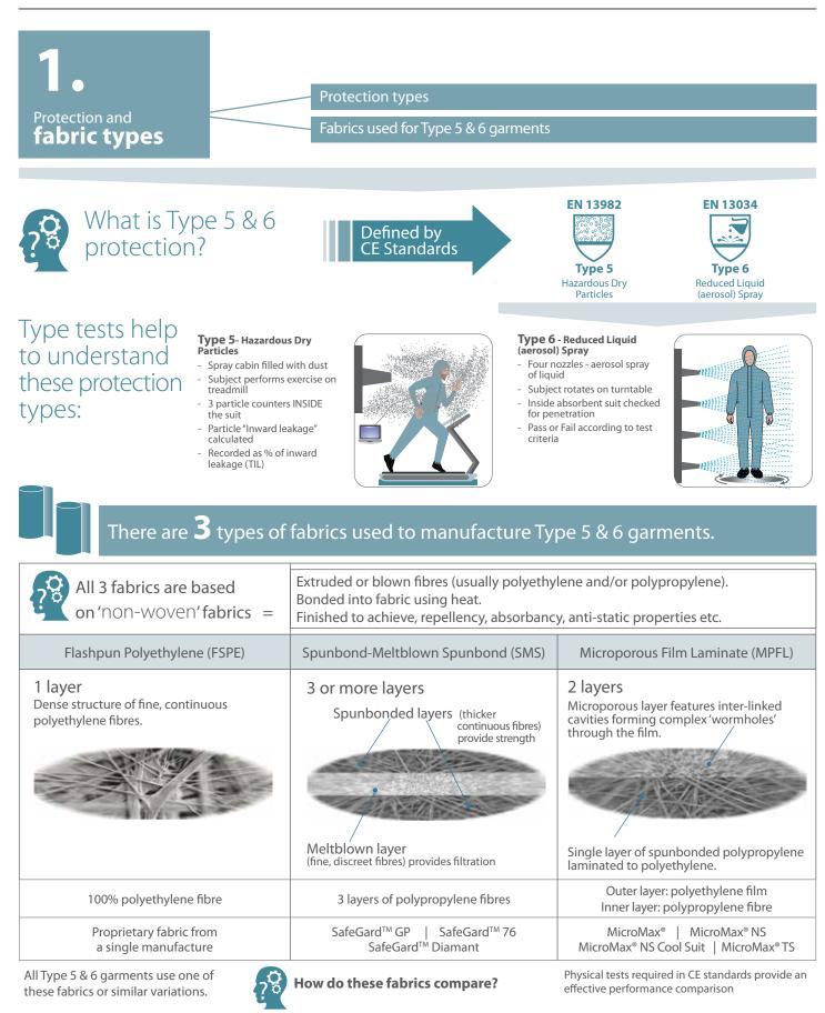
Note: All three fabrics have some level of porosity and are therefore not effective barriers to permeation of hazardous chemicals. More hazardous chemicals should be protected against using EN 14605 Type 3 & 4 chemical garments which are tested using a permeation test rather than the repellency test used for Type 6 garments. See the Lakeland Guide to Chemical Suit Selection
